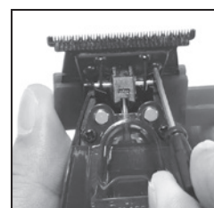
Step 6 – Once the blade is adjusted to zero gap or your liking, gently tighten the two screws on each side of the blade while holding the zero-gap tool in place. If the blade is not adjusted to satisfaction after testing, repeat the adjusting process.
