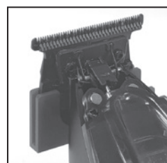
Step 5 – MAKE SURE THE MOVING CUTTING BLADE DOES NOT EXTEND PAST THE FIXED BLADE. WARNING: IF THE CUTTING BLADE EXTENDS PAST THE FIXED BLADE, YOU CAN POTENTIALLY CUT YOURSELF.
