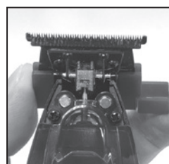
Step 4 – Using your fingers on each side of the zero-gap tool, push up until the cutting blade is even with or slightly below the black fixed blade.
